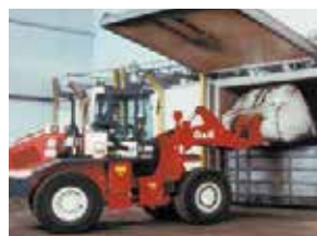
Filling of Herhof composting box by wheel loader
